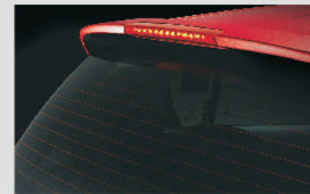
Rear Spoiler The rear spoiler with an integrated stop lamp, lends an aerodynamic and sporty appeal to the car.
