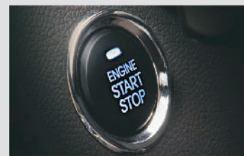
Push Button Start / Stop System The start / stop button allows you to turn the engine on and off at the touch of a button.
