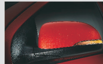
Electric Mirrors with Turn Indicator Electrically adjustable and foldable ORVMs maximize driver comfort while the turn indicators lend a premium touch and provide enhanced safety.
