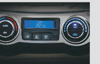
Fully Automatic Temperature Control The AC allows you to set the temperature and the system takes over to ensure uniform and convenient cooling at all times.
